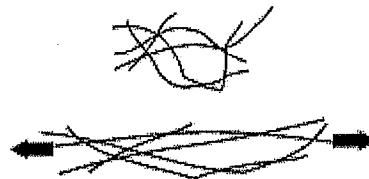
Fig. 3a elastic bands are made of a tangle of chain-like molecules
